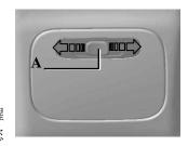
If regulating button A to door gear, inside lamp will be lit up to remind the user when the door is open or is not closed. The user may regulate button A to door gear; this lamp will be lit up when the user gets on or off the vehicle. Meanwhile, inside lamp will be lit up to remind the user when the door is open or is not closed.
